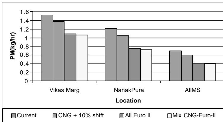
**FIGURE 2d Comparison of PM emissions under various scenarios of bus fuels with 10% shift to 2-wheelers in case of CNG.**
