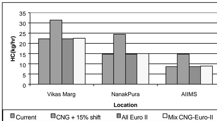
**FIGURE 3b Comparison of HC emissions under various scenarios of bus fuels with 15% shift to 2-wheelers in case of CNG.**
