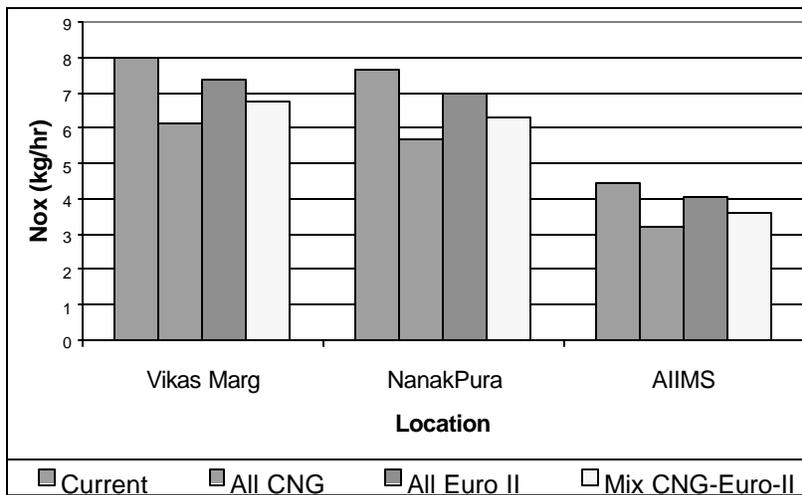
**FIGURE 1c Comparison of NOx emissions under various scenarios of bus fuels without shift to 2-wheelers.**
