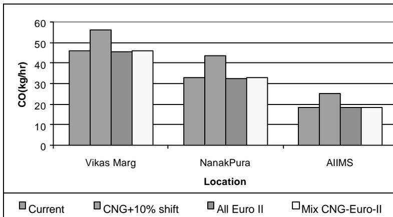
**FIGURE 2a Comparison of CO emissions under various scenarios of bus fuels with 10% shift to 2-wheelers in case of CNG.**
