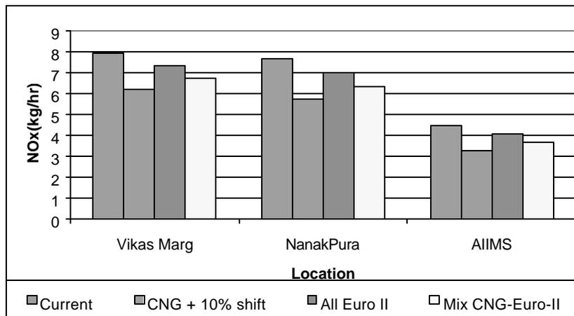
**FIGURE 3c Comparison of NOx emissions under various scenarios of bus fuels with 15% shift to 2-wheelers in case of CNG.**
