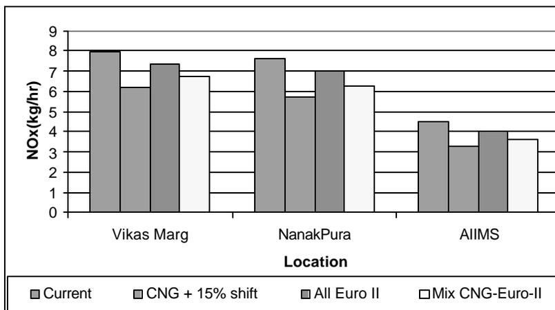
**FIGURE 2c Comparison of NOx emissions under various scenarios of bus fuels with 10% shift to 2-wheelers in case of CNG.**
