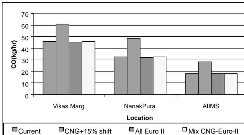
**FIGURE 3a Comparison of CO emissions under various scenarios of bus fuels with 15% shift to 2-wheelers in case of CNG.**
