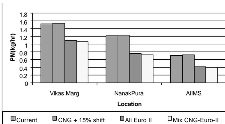
**FIGURE 3d Comparison of PM emissions under various scenarios of bus fuels with 15% shift to 2-wheelers in case of CNG.**
