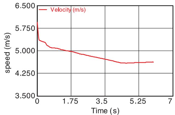
**Figure 17 :** Speed of RTV with Unrestrained Passengers in the Simulations for J-Turn Maneuvers
