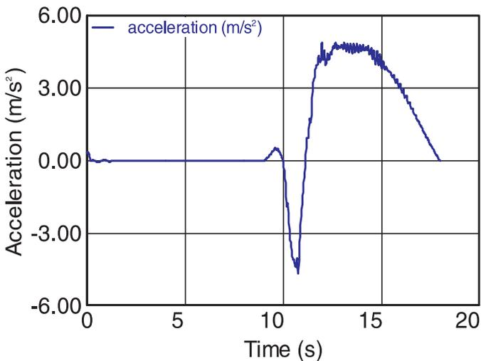
**Figure 19** : Lateral Acceleration of RTV without Passengers for RER Maneuvers
