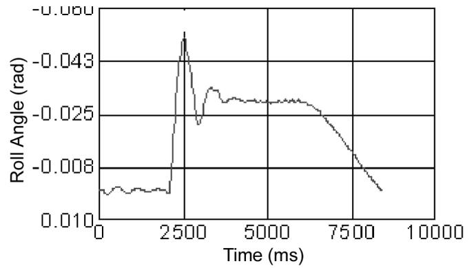
**Figure 10** : Roll Angle of RTV without Passengers
