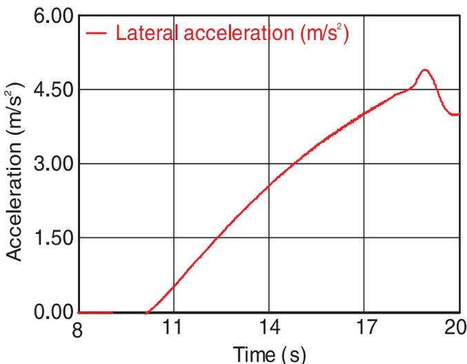
**Figure 6** : Lateral Acceleration in the Simulation for SIS Maneuvers
