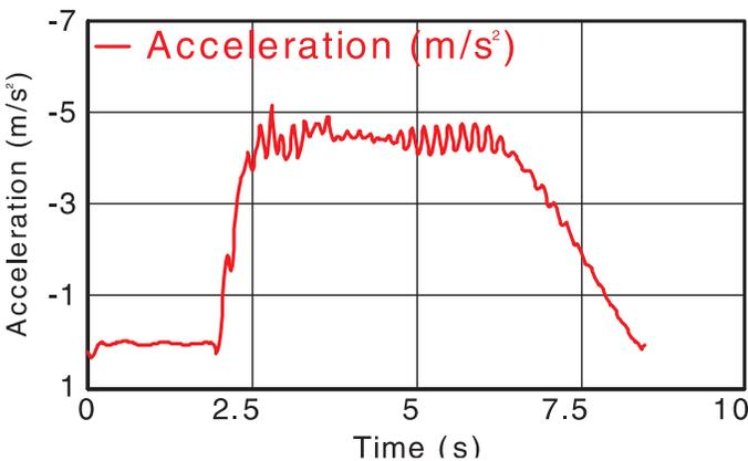
**Figure 9** : Lateral Acceleration of RTV Without Passengers
