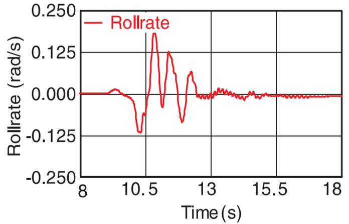
**Figure 21** : Roll Rate of RTV without Passengers for RER Maneuvers
