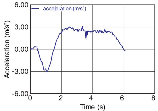
**Figure 27** : Lateral Acceleration of RTV with Unrestrained Passengers for RER Maneuvers
