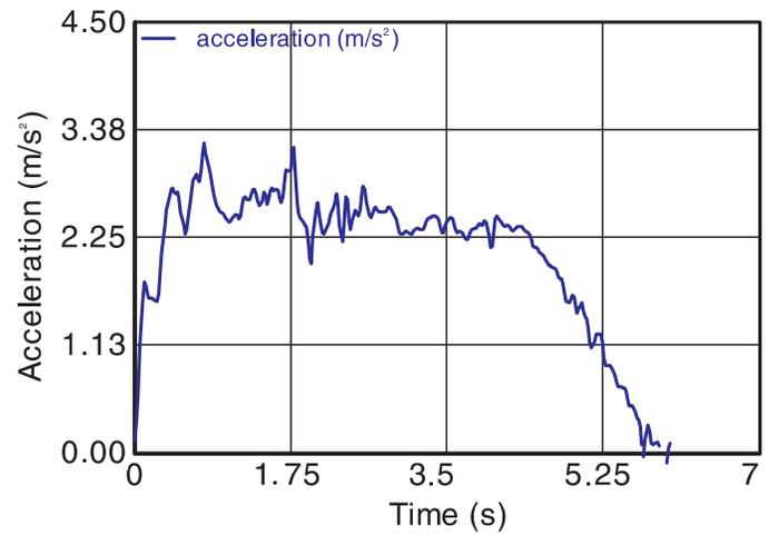
**Figure 16 :** Lateral Acceleration of RTV with Unrestrained Passengers for J-Turn Maneuvers
