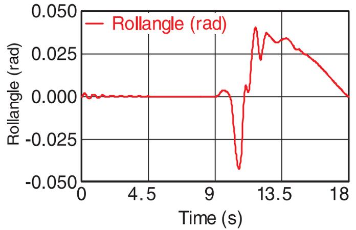
**Figure 20** : Roll Angle of RTV without Passengers for RER Maneuvers
