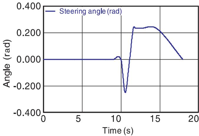
**Figure 18** : Steering Input in Simulation for RER Maneuver
