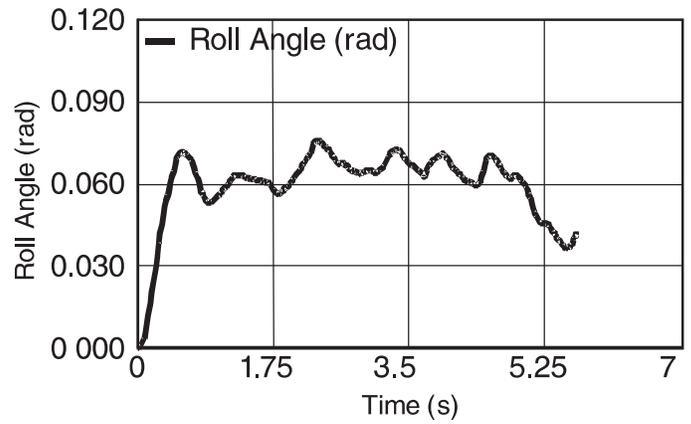
**Figure 15 :** Roll Angle of RTV with Unrestrained Passengers for J-Turn Maneuvers
