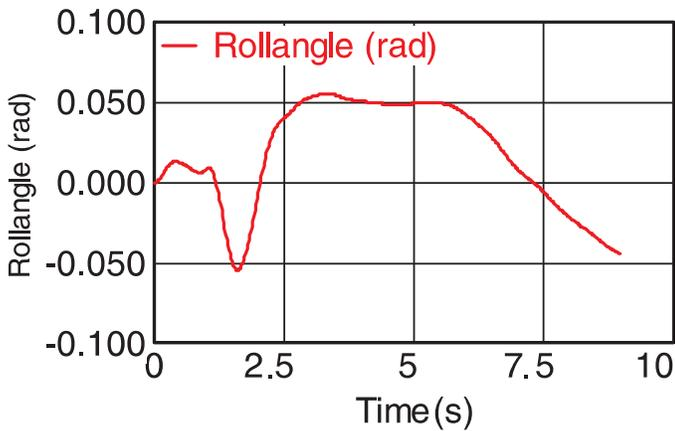
**Figure 24** : Roll Angle of RTV with Restrained Passengers for RER Msaneuvers
