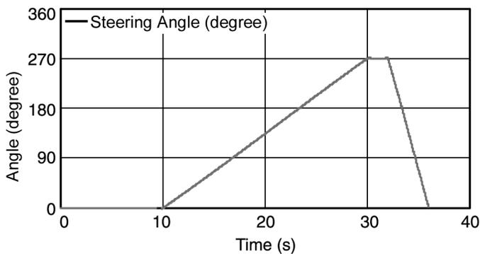
**Figure 5** : Steering Input in the Simulation for SIS Maneuvers
