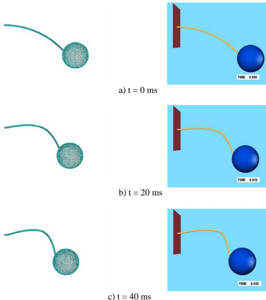
Fig. 4 - Comparison of FE (left) and MB (right) cantilever shape at peak deflection for three impacts
