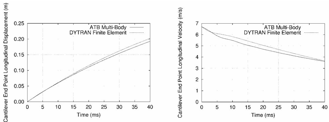
Fig. 2 - Comparison of MB and FE time histories for cantilever end longitudinal deflection and velocity for 13.7 m/s span-wise impact
