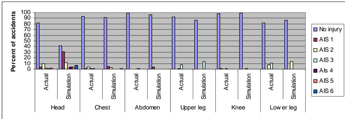
Fig. 1 - Comparison of simulated and real injury severities for n=501 LA/Hannover accidents by body region
