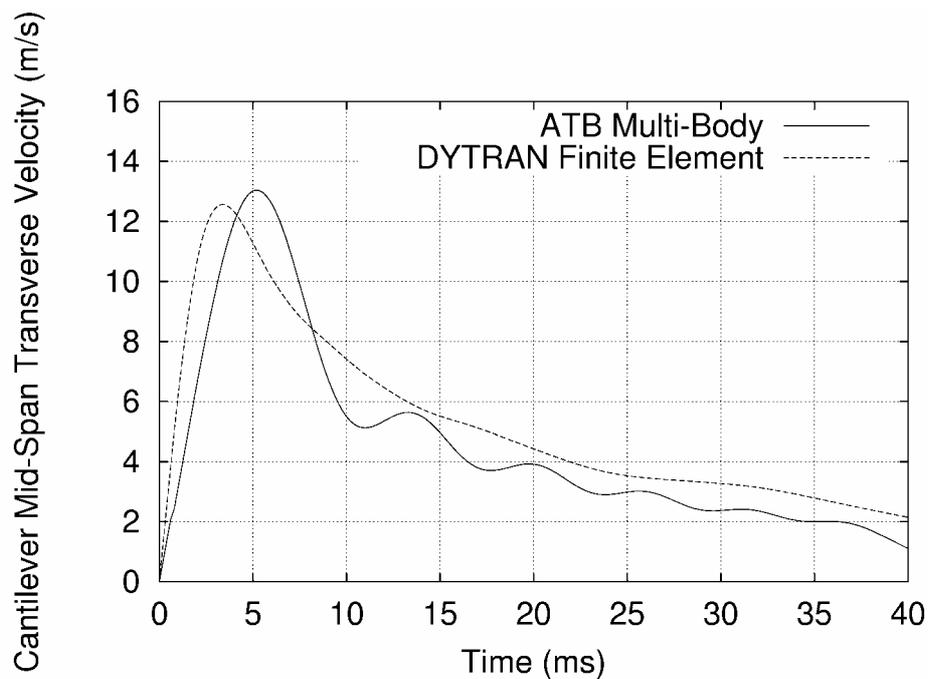
Fig. 3 - Comparison of MB and FE time histories for cantilever mid-span transverse velocity for 13.7 m/s span-wise impact
