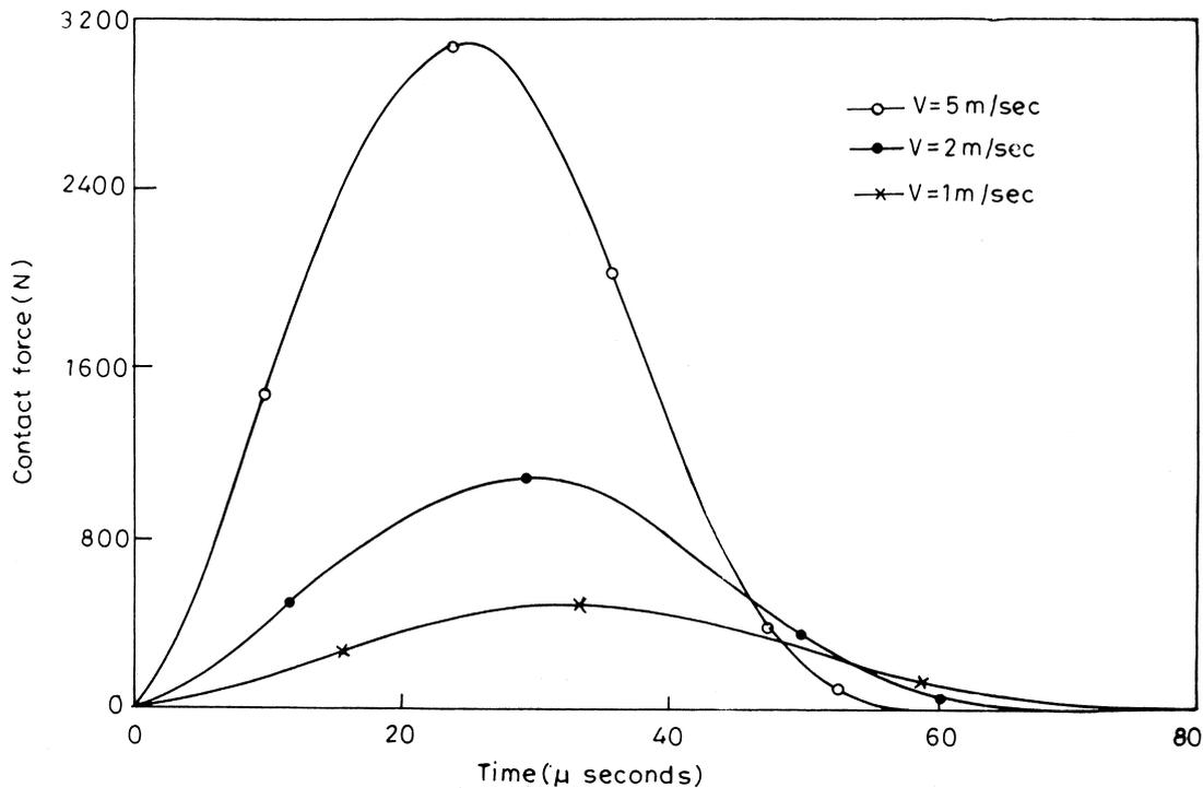
Fig. 9. Contact force (point contact) vs time for different impact velocity but fixed  $m_I/m_P$ .
