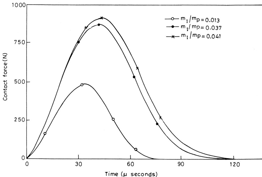
Fig. 10. Contact force (point contact) vs time for constant impact velocity but different  $m_I/m_P$ .
