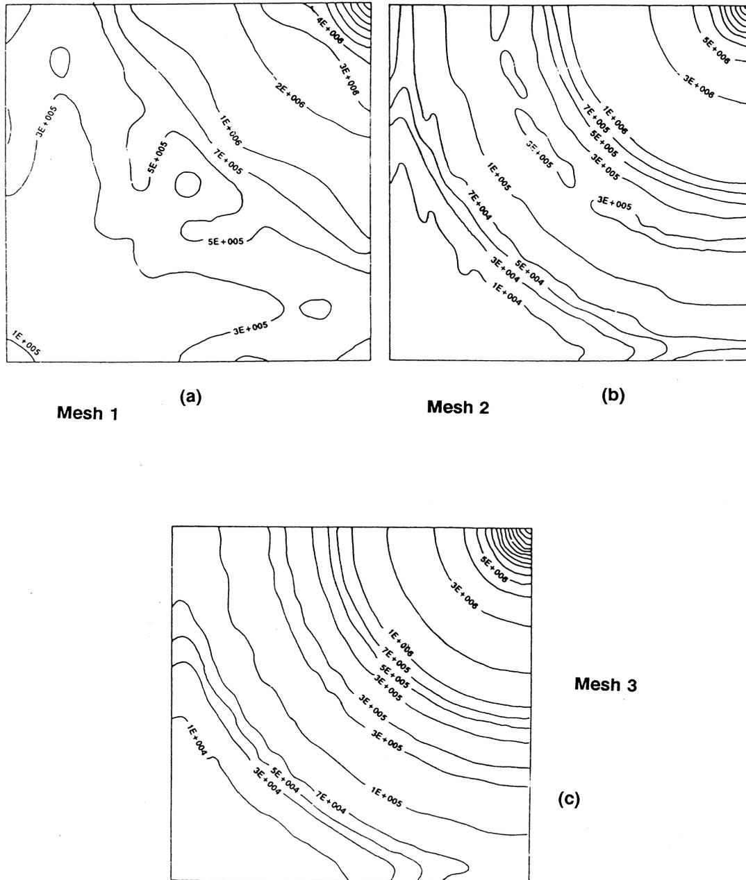
**EFFECTIVE STRESS (N/M<sup>2</sup>) CONTOURS OF TARGET PLATE IMPACTED BY SPHERICAL IMPACTOR**
