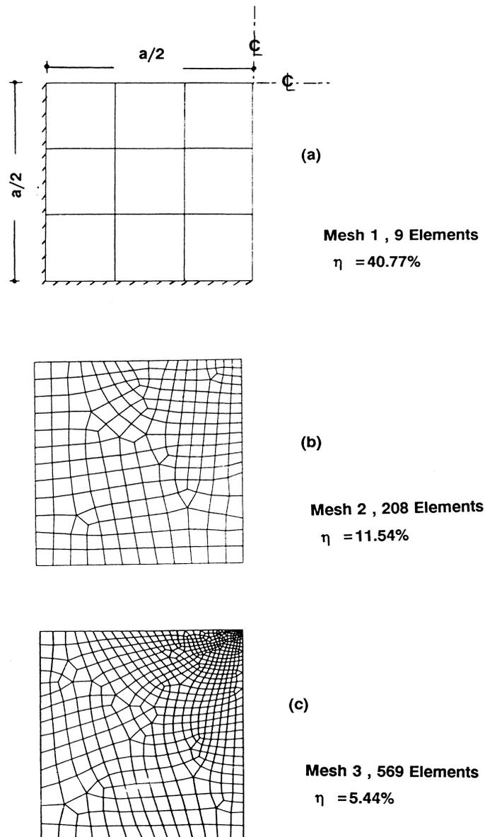
Fig. 3. Symmetric quadrant of clamped square plate ( $a/t = 25$ ) subjected to impact by a sphere at the centre of the plate.
