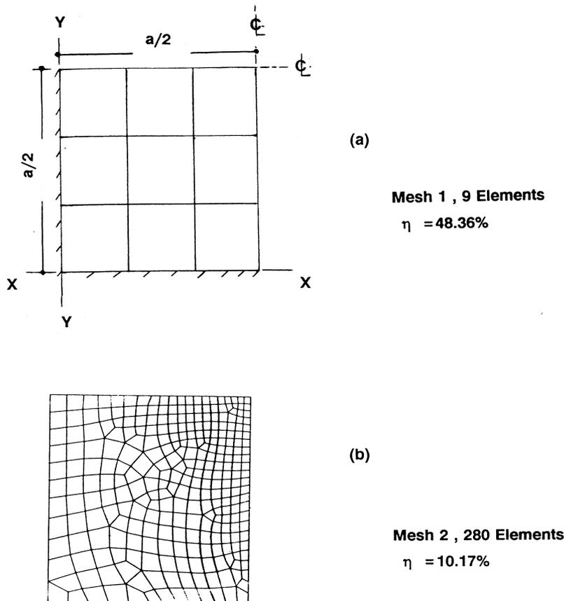
Fig. 6. Symmetric quadrant of clamped square plate ( $a/t = 25$ ) subjected to impact by a cylinder along central line (parallel to  $XX$ ) of the plate.
