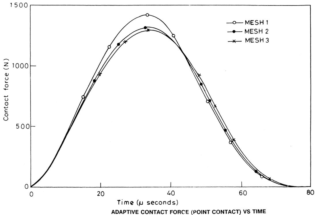
Fig. 4. Adaptive contact force (point contact) vs time.
