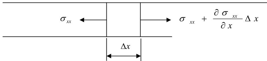
Fig. 3- Schematic of an element in a SHPB
