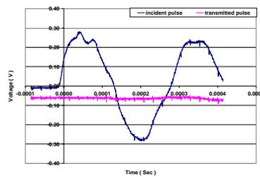
Fig. 6- Typical pulse obtained from strain gauges
