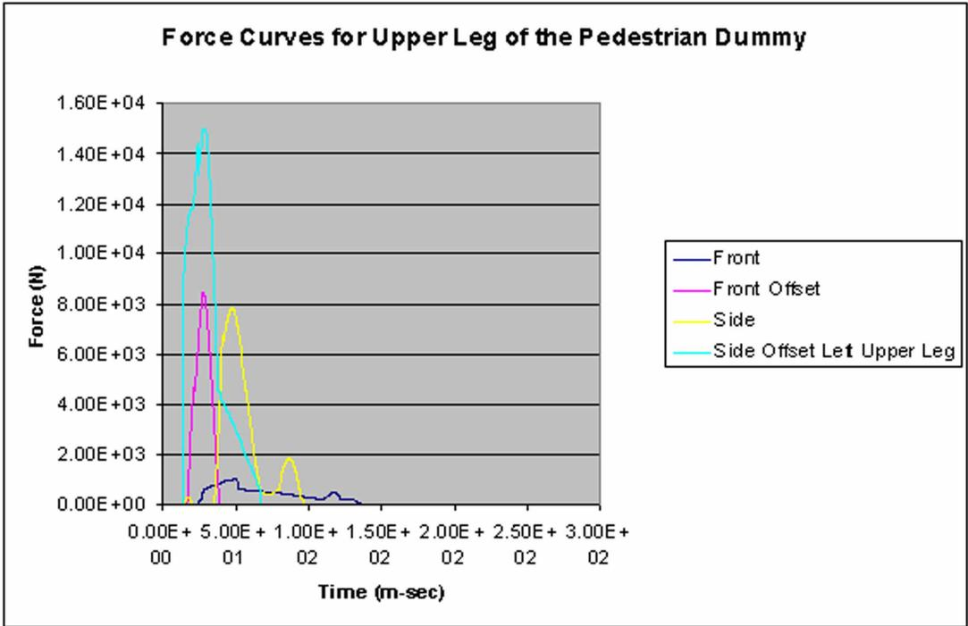
Figure 10 Acceleration curve for Upper Leg of the Pedestrian Dummy for the four pedestrian impact simulations.
