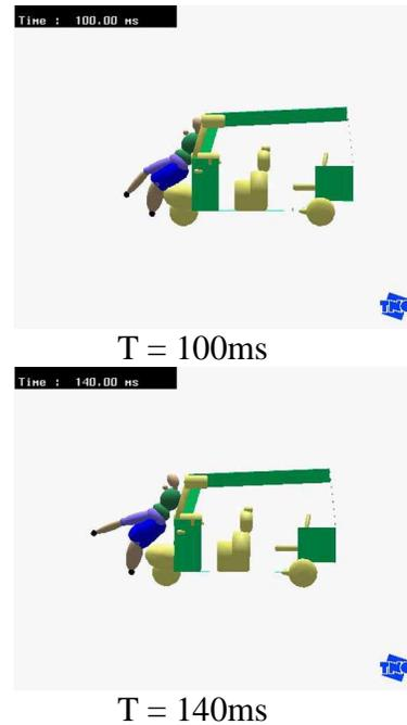
Figure 7 Kinematics for the Case III simulation
