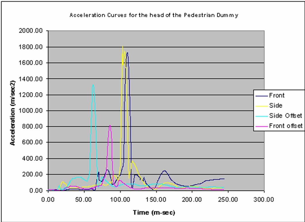
Figure 11 Acceleration curve for the Head of the Pedestrian dummy for the four pedestrian impact simulations.
