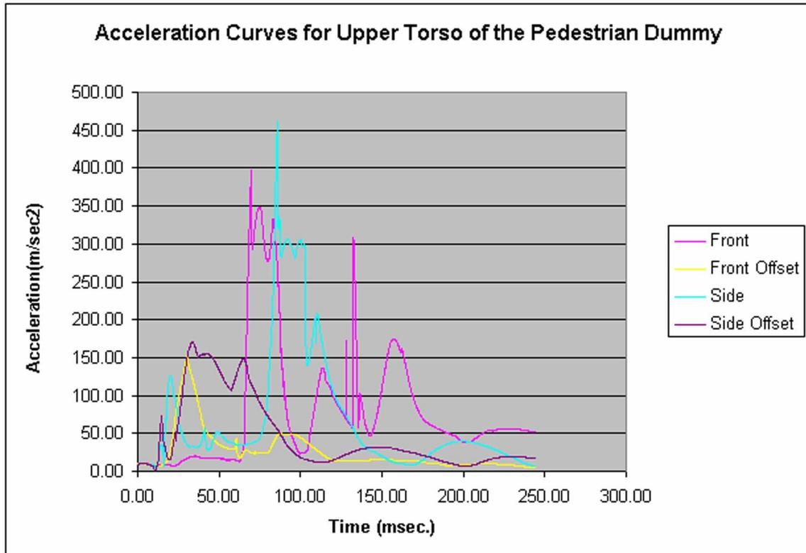
Figure 9 Acceleration curve for Upper Torso of the Pedestrian dummy for the four pedestrian impact simulations.
