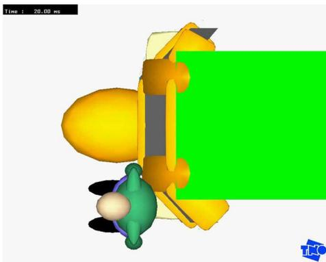
Figure 2 Configuration for the Pedestrian – TST frontal impact simulation with offset (Case II)
