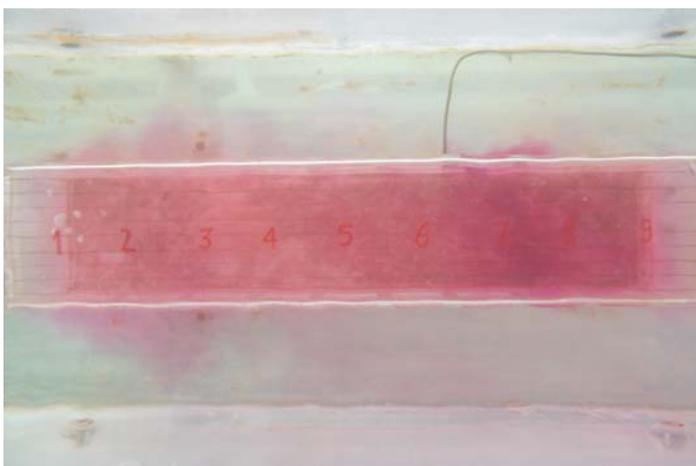
Air flow - bus with open window visualization at side center
