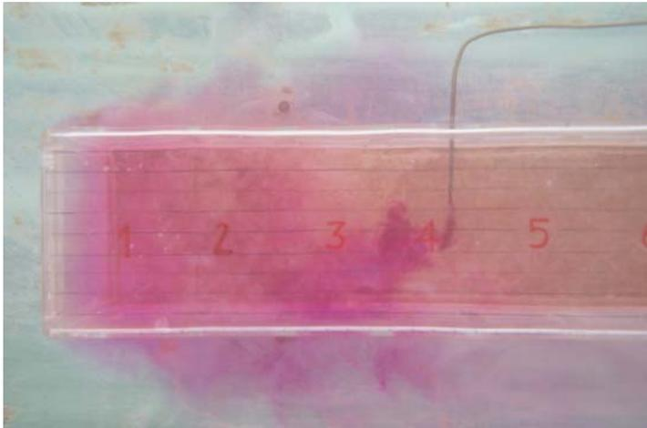
Air flow - bus with open window visualization inside bus middle
