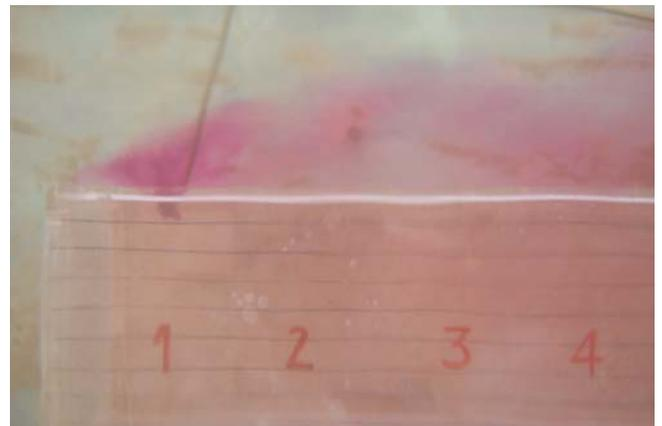
Air flow - bus with open window visualization at first window
