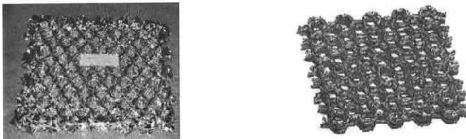
Figure 11.3 Crushing of honeycomb, test and simulation.
